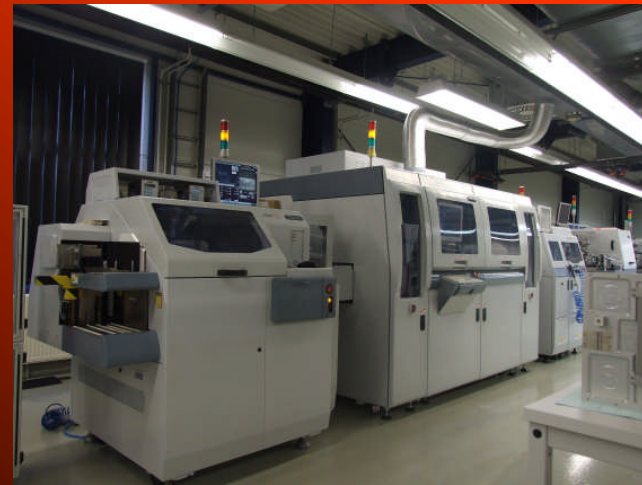
SMD LED encapsulation, singulation line: DS830+MC609H+IBE139H+MP- TAB+SLS230T+TLB203 and TLB400
