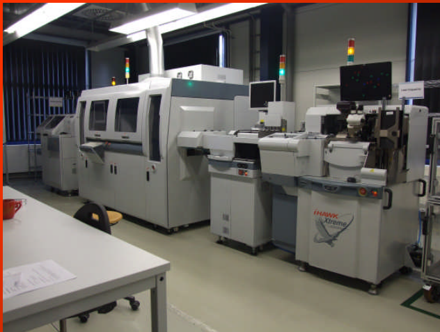
SMD LED bonding line: AD830+MC609H+IBE139H+iHawkXtreme
