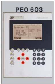
The standard furnace has a microprocessor based controller with digital outputs, 10 program locations of 100 steps each. Display and key pad are located on the front panel.
