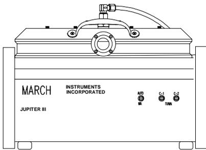
The top-loading chamber is designed to ensure anisotropic etching and maximize selectivity, uniformity, and speed. A ceramic ring focuses the plasma on the bottom electrode where the sample is placed, thus optimizing power utilization to increase anisotropy and etch rate. The bottom electrode is water cooled to maintain the sample at a low temperature during processing. The chamber is equipped with a circular quartz viewing window for
