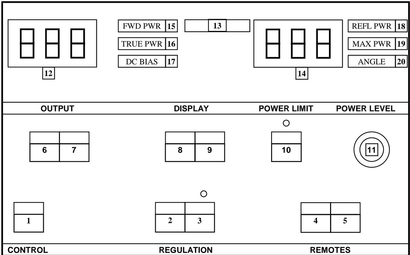
1. **POWER** - Applies power to internal circuitry. LED off = power off, LED on = power on.
