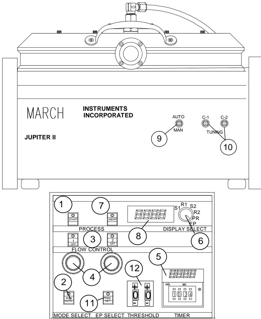
**FIGURE 3.- Process Controls and Indicators**
