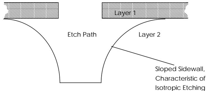
**Isotropic:** Etching that is not directional in its effect. Characteristic of most cleaning applications where it is desirable to remove material from all surfaces. Typical of barrel type etchers.
