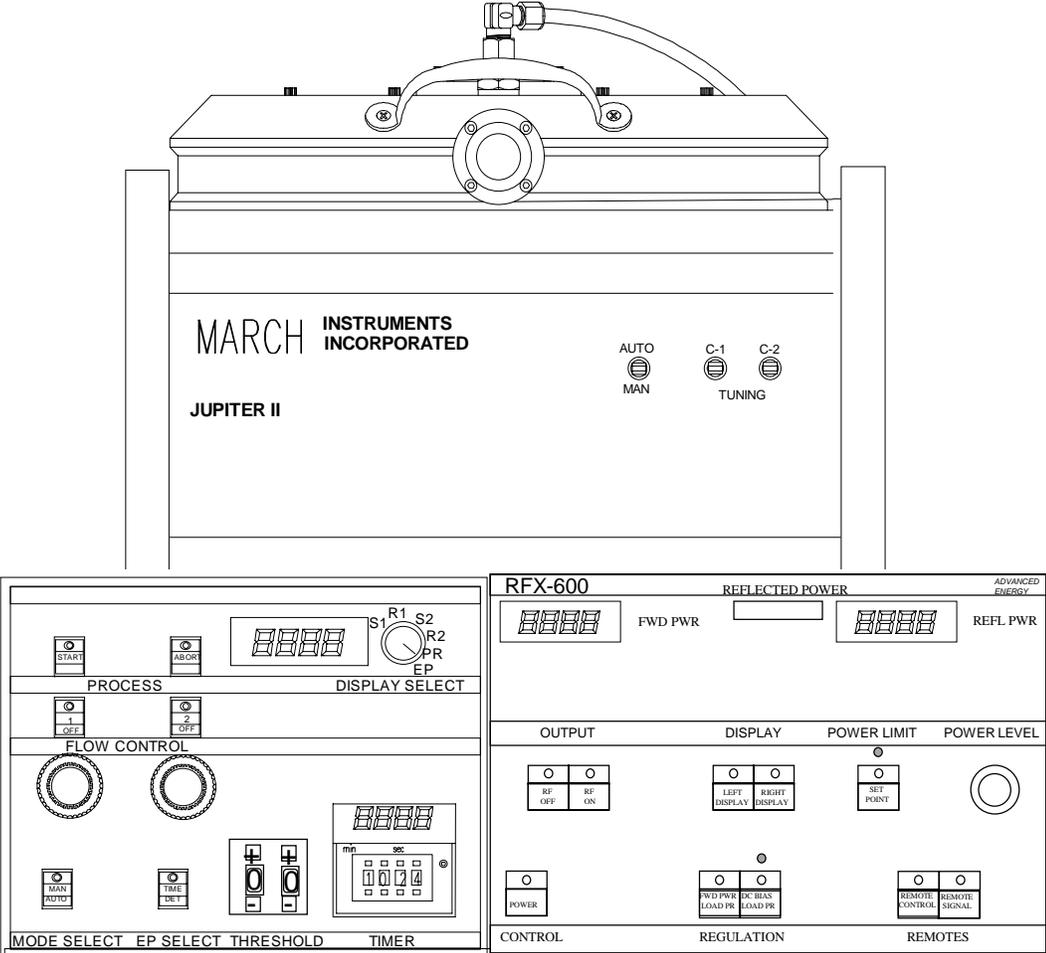
Designed for maximum performance and flexibility, March Instrument's Jupiter II Reactive Ion Etching systems are tabletop etchers used primarily in failure analysis and small scale production plasma etching applications.
