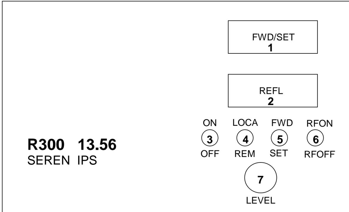
1. **FWD/SET Display** - Displays forward power output or forward power set point in the range of 0-300 watts
