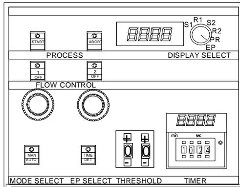
The Process Controller monitors and regulates the variable parameters of the plasma process, including chamber pressure, process duration and gas flow rates. The Process Controller houses two (or an optional four) Mass Flow Controllers for regulation of process gas flow, and the system is equipped with a Baratron pressure gauge for pressure determination.
